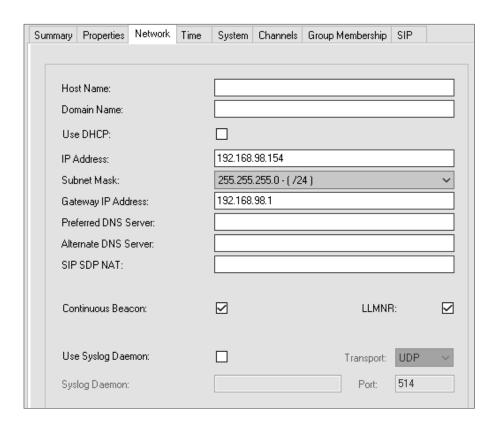
The **Network** tab contains fields to configure the **IP address** statically or check the "**Use DHCP**" box to acquire an IP address from a DHCP server on the network.
