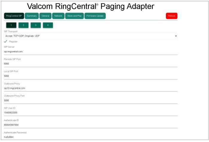
The **SIP tab** provides fields to configure the basic settings to allow this device to register with RingCentral. The entries are labeled similar to the names used in the RingCentral provisioning web pages.
