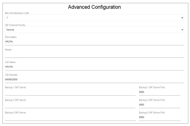
**Max Simultaneous Calls** indicates the number of calls allowed on this SIP channel before returning a busy signal. Leave on the default of 1 for RingCentral.
