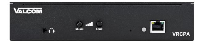
Valcom's VRCPA RingCentral® Page Adapter is designed to provide access to paging systems from RingCentral hosted Session Initiation Protocol (SIP) voice over IP (VoIP) connections, or through analog trunk or station inputs (FXO/FXS). When paired with RingCentral SIP connections the VRCPA supports Valcom handsfree page units for talkback paging and up to 150 Valcom one-way amplified speakers. The VRCPA can connect multiple units for multi-zone paging.
