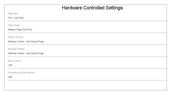
The second half of this screen shows configuration settings of the device. These fields indicate the settings of the hardware switches and volume control knobs on the VRCPA.
