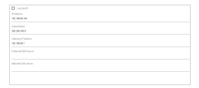
If the Use DHCP checkbox is <u>not</u> checked, the IP address information can be entered as static values. The web page will display fields for the **IP Address**, **Subnet Mask** and **Gateway IP Address**. The fields for **DNS Server** entries are optional, although other programming options for SIP may require the DNS entries to be entered.
