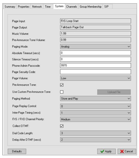
The **System** tab is where most of the device-specific capabilities are configured.
