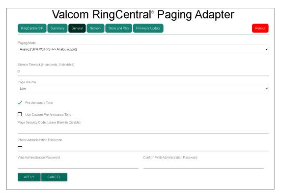
The **General** page includes settings for the Absolute Timeout (0-3600) and the **Silence Timeout** (0-600) in number of seconds (If DIP switches 2-5 are ON). Entering 0 for either disables that timeout. If **Store and Play** is active then Absolute Timeout is not configurable or displayed.
