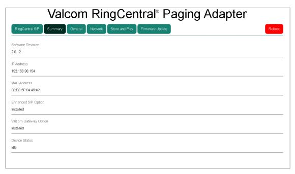
All of the fields on the Summary page are read-only, and reflect the current status of the VRCPA. The first section of the screen displays property information about the device.
